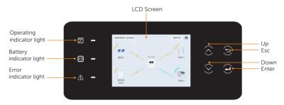
Figure 10-1 Control Panel of the inverter
