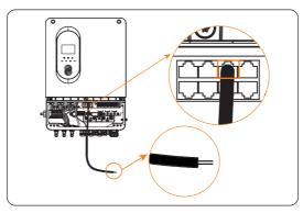
Figure 8-49 Inserting the cable into the Meter/CT port
