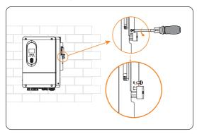
Figure 13-3 Unscrewing the M4 screws
