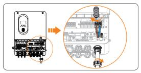
Figure 8-23 Connecting the GRID cable
