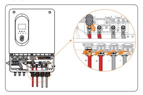
Figure 13-2 Removing the battery connector
