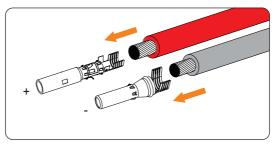
Figure 8-25 Inserting the PV pin contact
