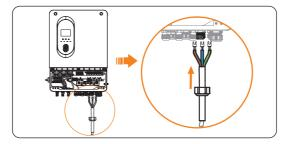
Figure 8-16 Threading the GEN cable
