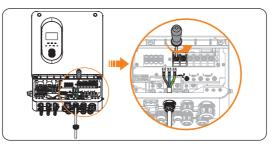
Figure 8-18 Loosening the EPS screws
