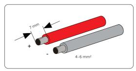
**Step 1:** Strip the insulation of the PV cables to an appropriate length.
