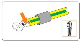
Figure 8-4 Crimping the cable
