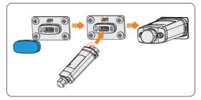
Figure 8-67 Dongle connection procedure
