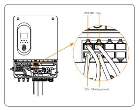
Figure 8-59 Connecting the DI/COM, BMS, DO, DRM port
