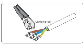
Figure 8-9 Crimping the conductors
