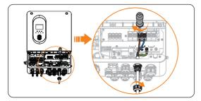
Figure 8-22 Connecting the GEN cable
