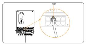
Figure 8-42 Inserting the cable into BMS port
