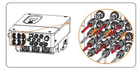
Figure 8-31 Connecting the PV cable
