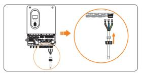
Figure 8-17 Threading the GRID cable
