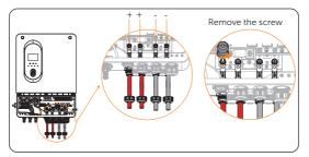
Figure 8-39 Removing the screws
