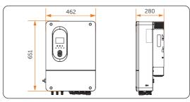
Figure 7-3 Dimensions 1 (Unit: mm)
