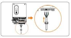
Figure 8-15 Threading the EPS cable
