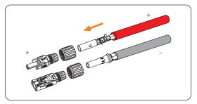
Figure 8-27 Threading the PV cable
