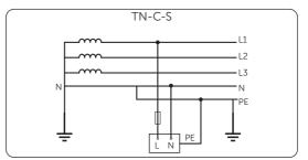
Figure 2-4 Supported power grid-TN-C-S
