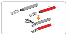
Figure 8-35 Inserting the battery connection terminal
