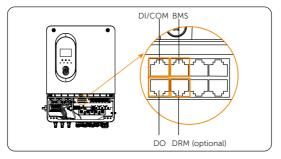
Figure 8-58 Finding the DI/COM, BMS, DO, DRM port
