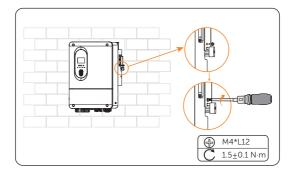
**Step 5:** Use M4\*12 screws (Part K) to secure the inverter on both sides.
