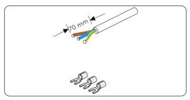
Figure 8-7 Stripping cables
