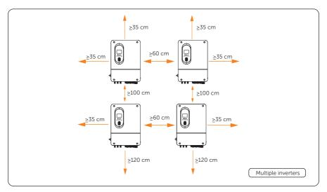
Figure 5-5 Clearance requirement for multiple inverters
