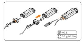
Figure 8-69 Assembling the dongle
