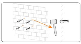
Figure 7-7 Knocking the expansion tubes
