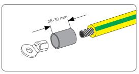
Figure 8-3 Installing the tubing and OT terminal
