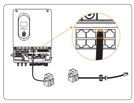
Figure 8-51 Inserting the cable into the Meter/CT port
