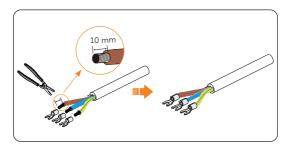
Figure 8-8 Stripping cables
