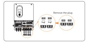
Figure 8-37 Removing the plug
