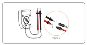
Figure 8-29 Measuring the voltage of PV connectors
