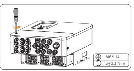
Figure 8-10 Loosening the screws
