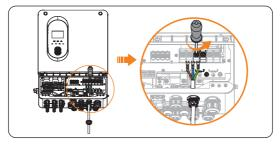
Figure 8-19 Loosening the GEN screws
