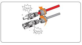
Figure 8-28 Securing the PV cable
