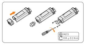
Figure 8-66 Assembling the dongle
