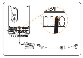
Figure 8-53 Inserting the cable into the Meter/CT port
