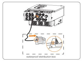
Figure 8-50 Inserting the cable into the Meter
