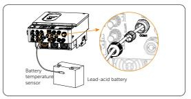
Figure 8-41 Disassemble the swivel nut and attaching the terminal
