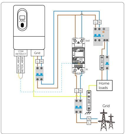
Figure 8-45 Meter connection diagram
