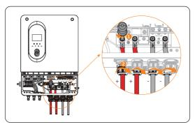
Figure 8-40 Connecting the battery connector
