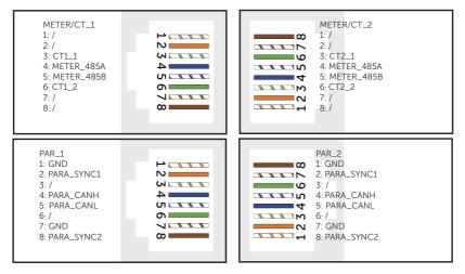
Figure 8-43 Pin assignment of COM terminal
