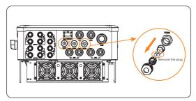
Figure 8-47 Removing the plug
