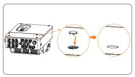
Figure 8-63 Installing the decorative buckles
