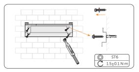
Figure 7-8 Securing the wall mounting bracket
