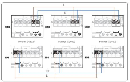
Figure 15-2 Power cable wiring
