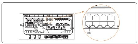
Figure 15-5 Connection terminal for generator
