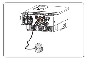
Figure 8-52 Tightening the swivel nut
