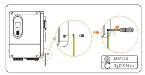
Figure 8-6 Securing the PE cable
