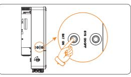
**Step 7:** Turn on the system button at the left side of the inverter, the light on the system button will light up. Then the inverter will start automatically.
