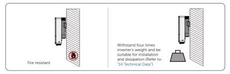
Figure 5-3 Installation carrier requirement
