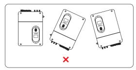
Figure 7-2 Incorrect installation
