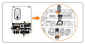
Figure 8-21 Connecting the EPS cable
