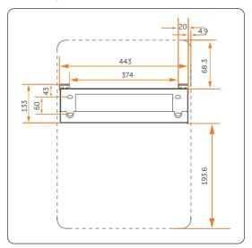
Figure 7-4 Dimensions 2 (Unit: mm)
