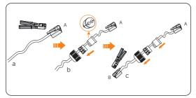
Figure 8-48 Crimping RJ45 terminal
