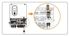
Figure 8-20 Loosening the GRID screws
