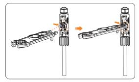
Figure 13-1 Disassembling the PV connector
