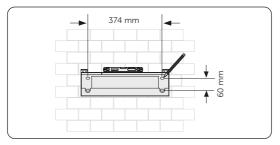
Figure 7-5 Marking the holes
