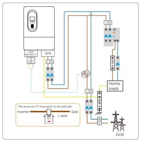
Figure 8-46 CT connection diagram
