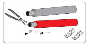
Figure 8-34 Stripping the battery cable
