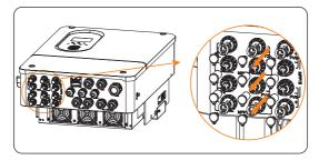
Figure 8-30 Removing the PV terminal caps
