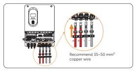
Step 4: Thread the battery cable through swivel nut and the battery terminal.
