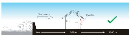
Figure 5-1 Recommended installation position
