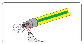
Figure 8-5 Shrinking the tubing
