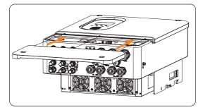
Figure 8-61 Put the lower cover back
