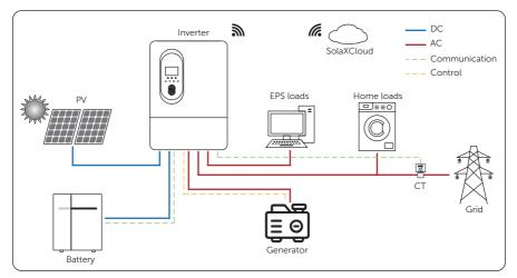
Figure 15-4 Dry contact wiring diagram
