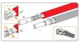
Figure 8-26 Crimping the terminal
