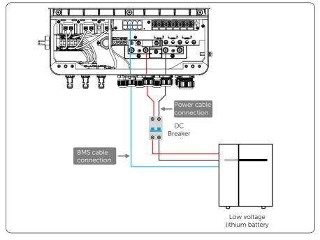
Figure 8-32 Lithium battery connection diagram
