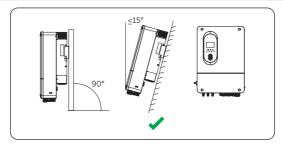
Figure 7-1 Correct installation
