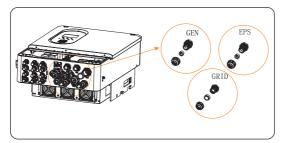
Figure 8-12 Removing the plugs
