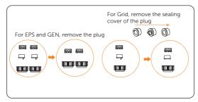
Figure 8-13 Removing the plugs
