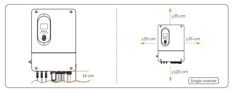
Figure 5-4 Clearance requirement for single inverter
