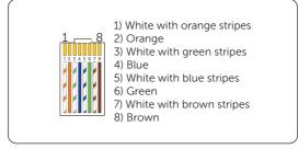
Figure 8-56 Pin order of RJ45 terminal
